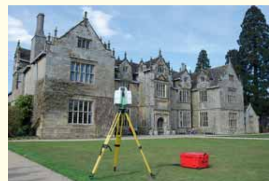
Fig CS7.1 Laser scanning Wakehurst Place using a Leica C10.
