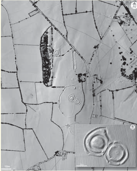
Fig CSII.1 Plan view of the DSM generated for the Hill of Tara from FLI-MAP data at approx. 60pts/m 2 (©The Discovery Programme).
