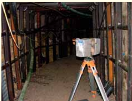
Fig CSI.1 (above) Faro LS880 protected for scanning.
