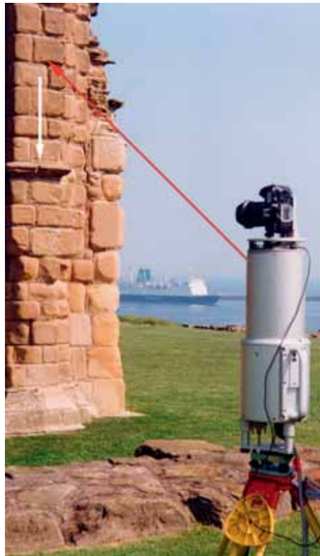
Fig 16 (above) A time-of-flight laser scanner, showing measurement beam and direction of scan (courtesy of Riegl UK)
