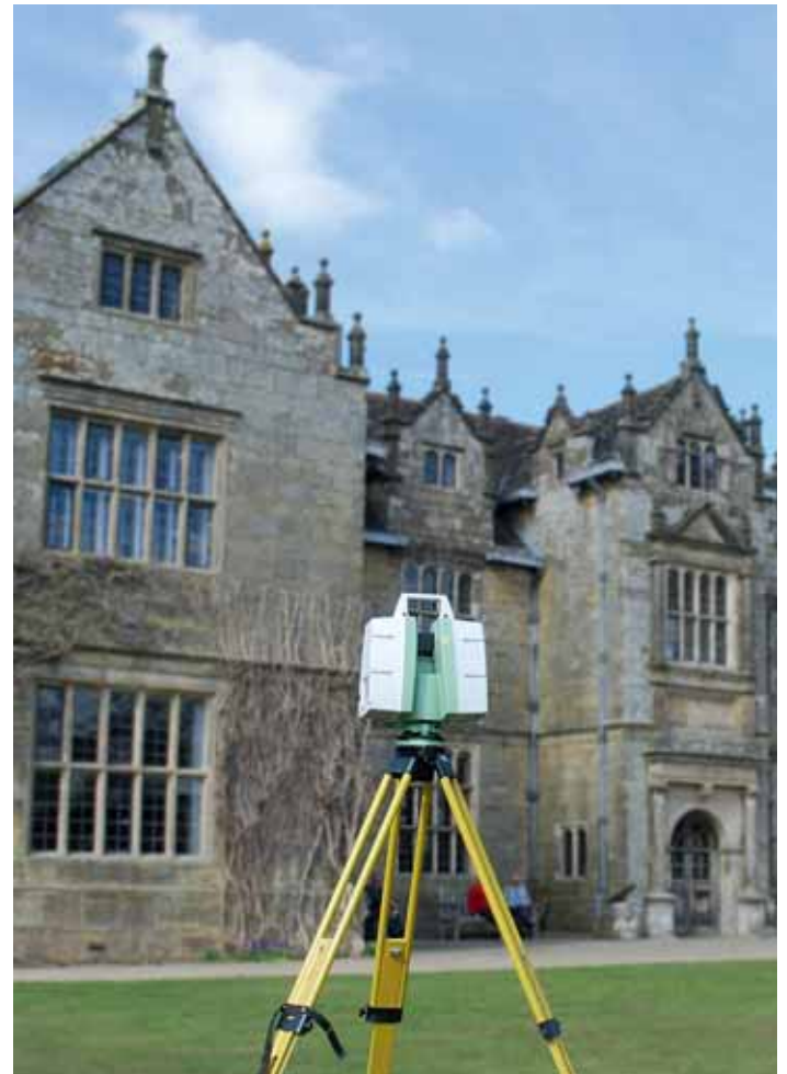
Fig 2 Triangulation laser scanning (courtesy of Conservation Technologies, National Museums Liverpool). Fig 3 Time-of-flight laser scanning (courtesy of Wessex Archaeology).
