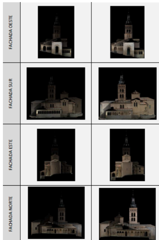
Fig. 9. Orthoimages of Saint Martin's Church façades.
