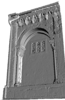
Fig. 5. Example of the creation of a mesh in an arcade of the church.
